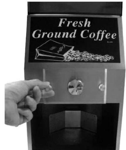
8. Set brew basket stop for size brew baskets being used. There are three basic sizes for the brew baskets: 7-½ inches, 7 inches, and 6 inches. This dispenser is set for a 7 inch brew basket. If you're using a different size of brew basket, remove the two screws holding the brew basket stop and move stop to the location corresponding to your brew basket size.
