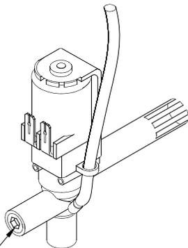
Adjust Water Flow Rate so that the water level reaches half way up in the Mixing Chamber, as shown.
